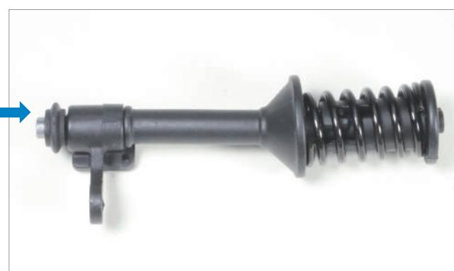
Fit the **Knuckle Arm (R) 15-D** and **Washer 15-C** onto the other end of **15-B**.
