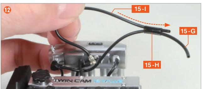
Thread Leads **15-G** and **15-I** through **Code Band 15-H** to bundle the two leads together.
