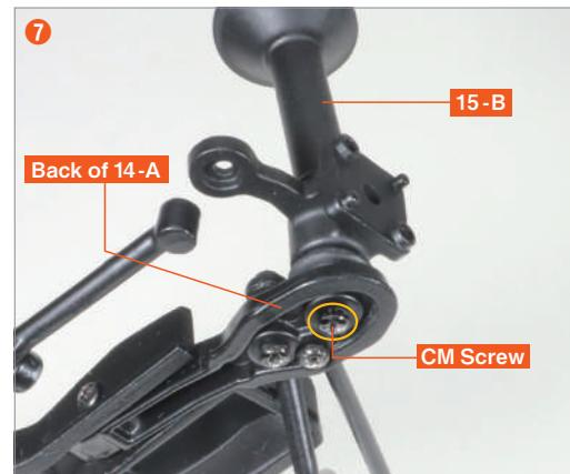
Turn the front axle over and fasten **14-A** from the back with a **CM screw**. Be careful not to tighten it too much, so that **15-B** can rotate freely.
