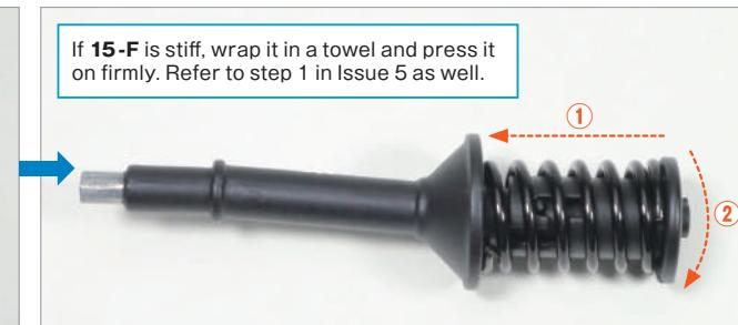
Slide the **Front Coil Spring 15-F** onto the end of the **MacPherson Strut (R) 15-B**, then fit the **Strut Upper Mount (R) 15-E**.
